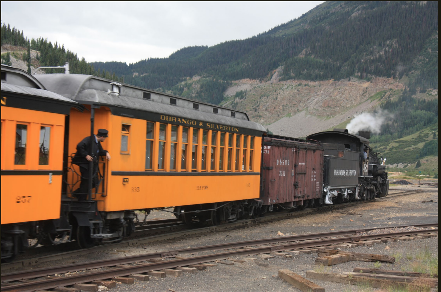
A conductor checks things out as a southbound Durango & Silverton train heads down Animas Canyon to Durango. Note the modern highway in the background, which ascends a ridge rather than deal with Animas Canyon, which is downhill all the way to Durango and the best route of a railroad. The track that veers right between the viewer and the train is the north branch of a turning wye.
