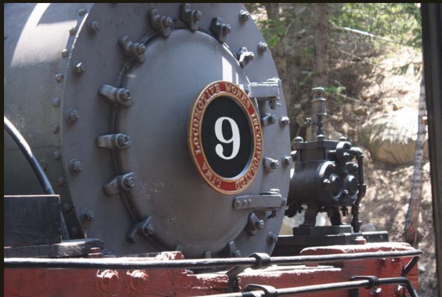
Georgetown Loop Railroad Engine #9, a narrow gauge Shay. Unlike the horizontal cylinders and rods that push the driver wheels on a standard steam engine, Shay locomotives have three vertical cylinders on one side of the boiler that drive a horizontal shaft with gears that drive every wheel on the locomotive and the tender, but only on one side of the engine (the side toward us).
