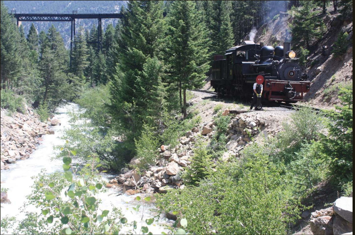
The Shay locomotive, just downstream from the Georgetown Station, switching to the siding so it can leap frog the to the other end of the train to pull it up to Silver Plume. Devil's Gate High Bridge in the distance.
