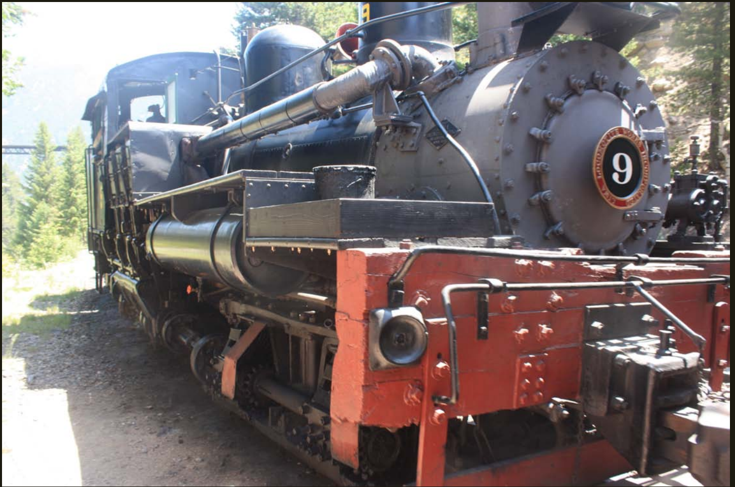
Georgetown Loop Railroad Engine #9, a narrow gauge Shay. Unlike the horizontal cylinders and rods that push the driver wheels on a standard steam engine, Shay locomotives have three vertical cylinders on one side of the boiler that drive a horizontal shaft with gears that drive every wheel on the locomotive and the tender, but only on one side of the engine (the side toward us).
