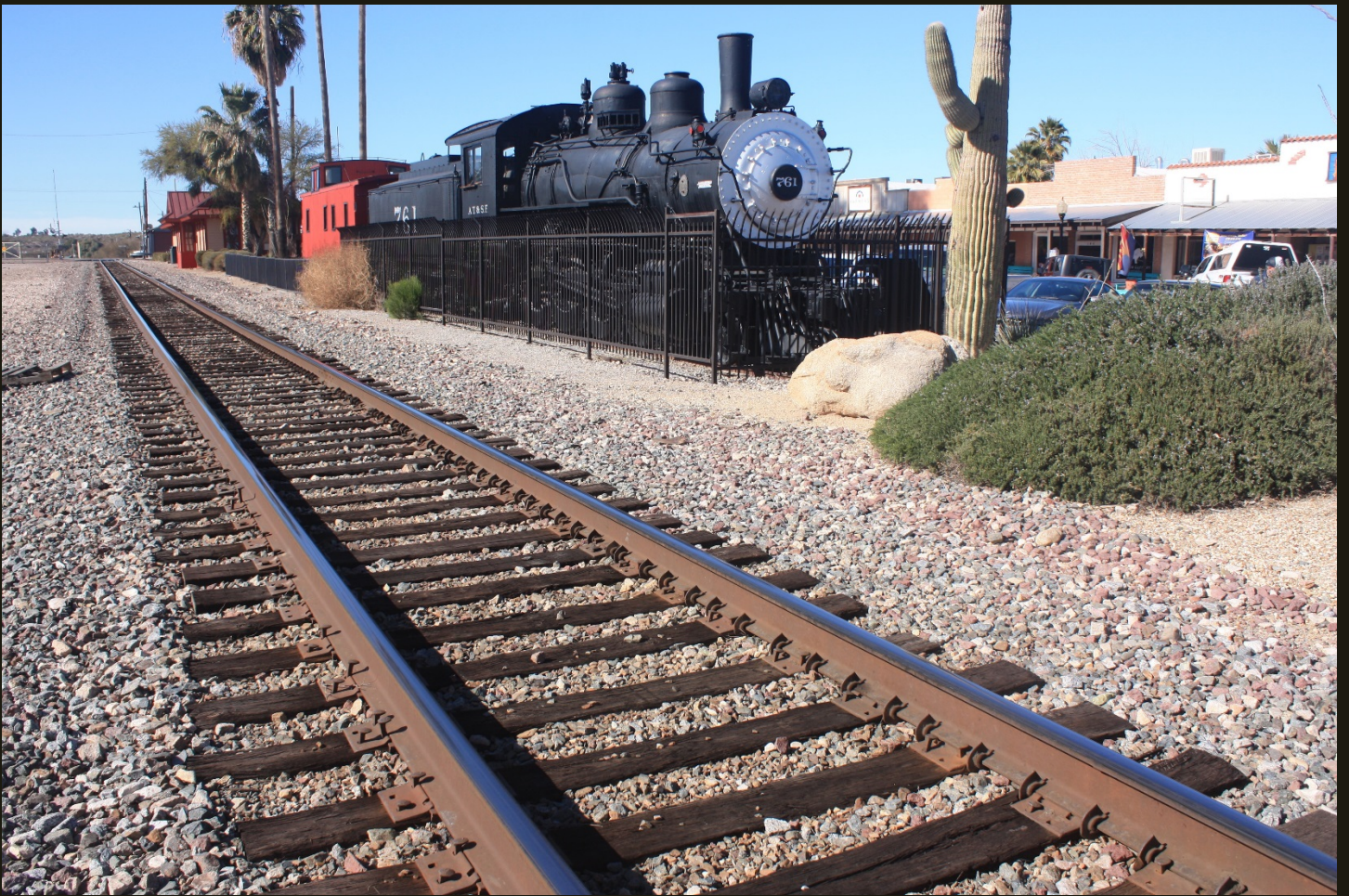
Northwestward view of the SFP&P (1895) at Wickenburg; the depot (previous photo) is just past the last palm tree in the left distance. AT&SF #761, a 2-8-0 built by Baldwin Locomotive Works in 1900, and other historical rolling stock are on display.
