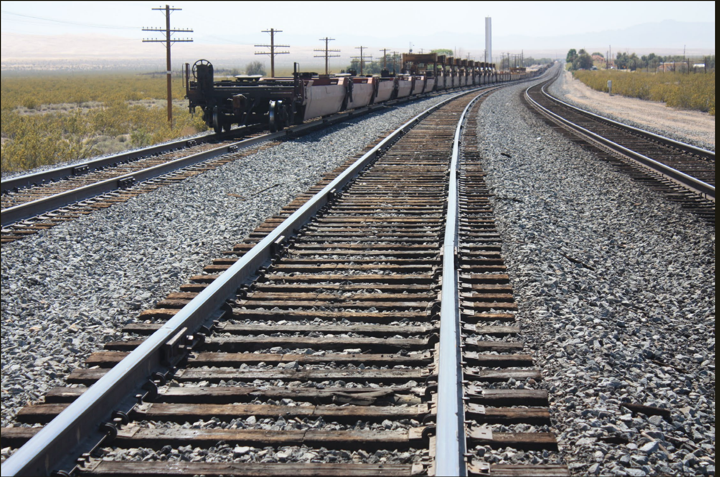
Southwestward view of container cars stored on Kelso sidings one mile northeast of Kelso. The depot is barely visible among the trees in the right distance. The mainline is on the far right, the only track with welded rails.
