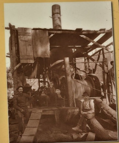
“Steam donkey” used for moving logs.
