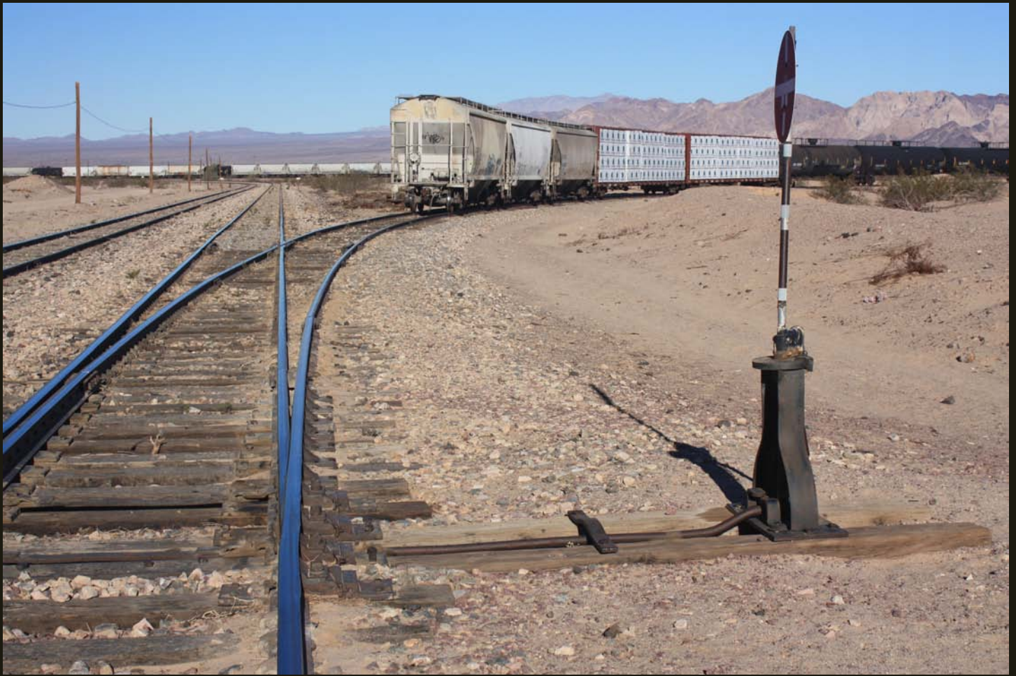
Northwestward view of the southern tip of the A&C wye, same location as previous. The double-tracked west branch of the A&C (1910) wye merges with the single-tracked east branch, used for car storage.
