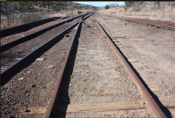
Southward view of the same SC&N switch at Cobre. The line to the left is active and services the open pit Chino mine and the track to the right is inactive and goes to a mine at Fierro; the central track is a siding. Note the gleaming active track to the Chino mine and the rusted track to Fierro.
