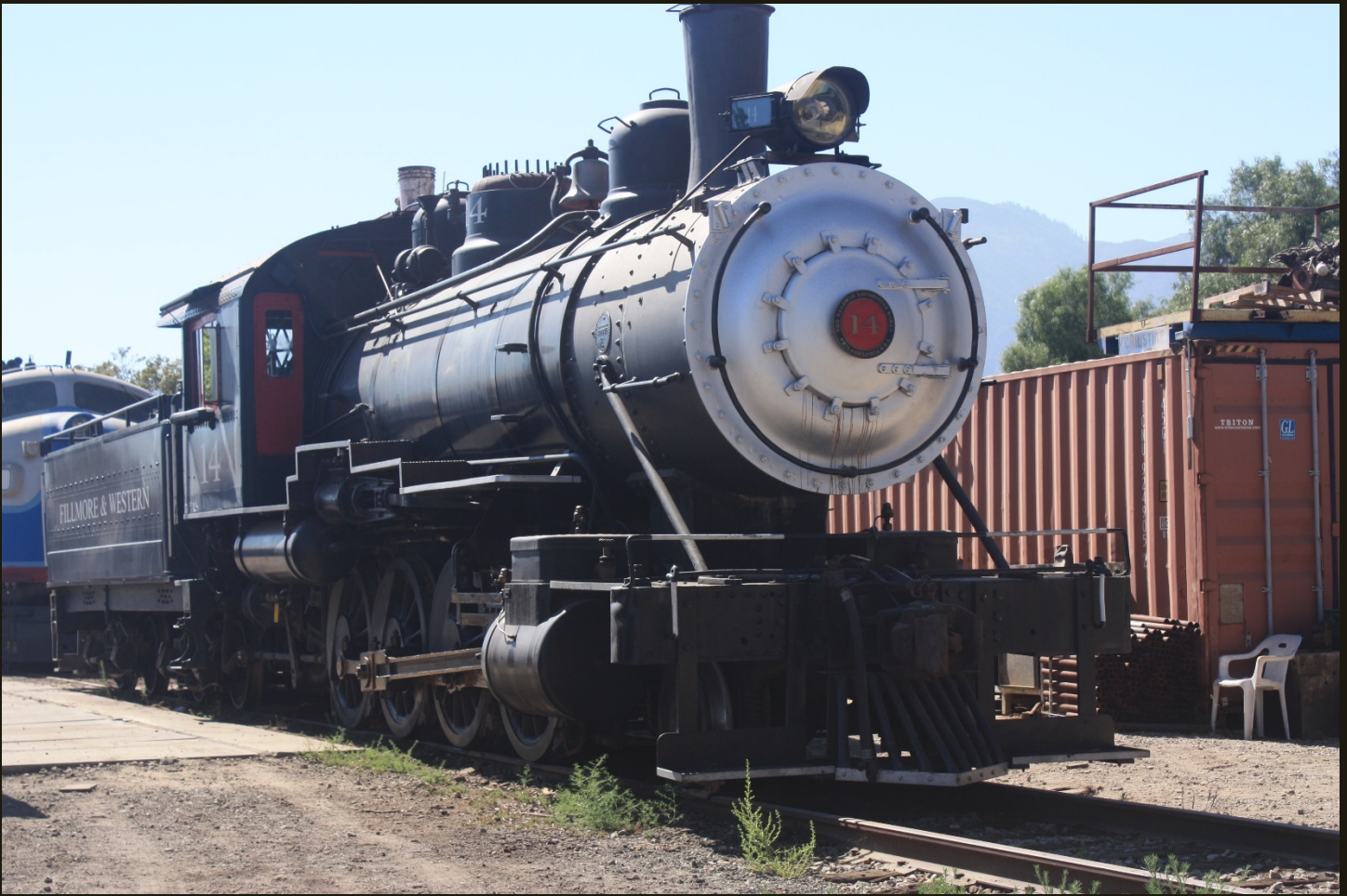
The F&W uses this operational steam locomotive in movies and to pull excursion trains. The F&W #14 is a 2-8-0 built by the Baldwin Locomotive Works in 1913 for the Duluth & Northeastern Railroad.
