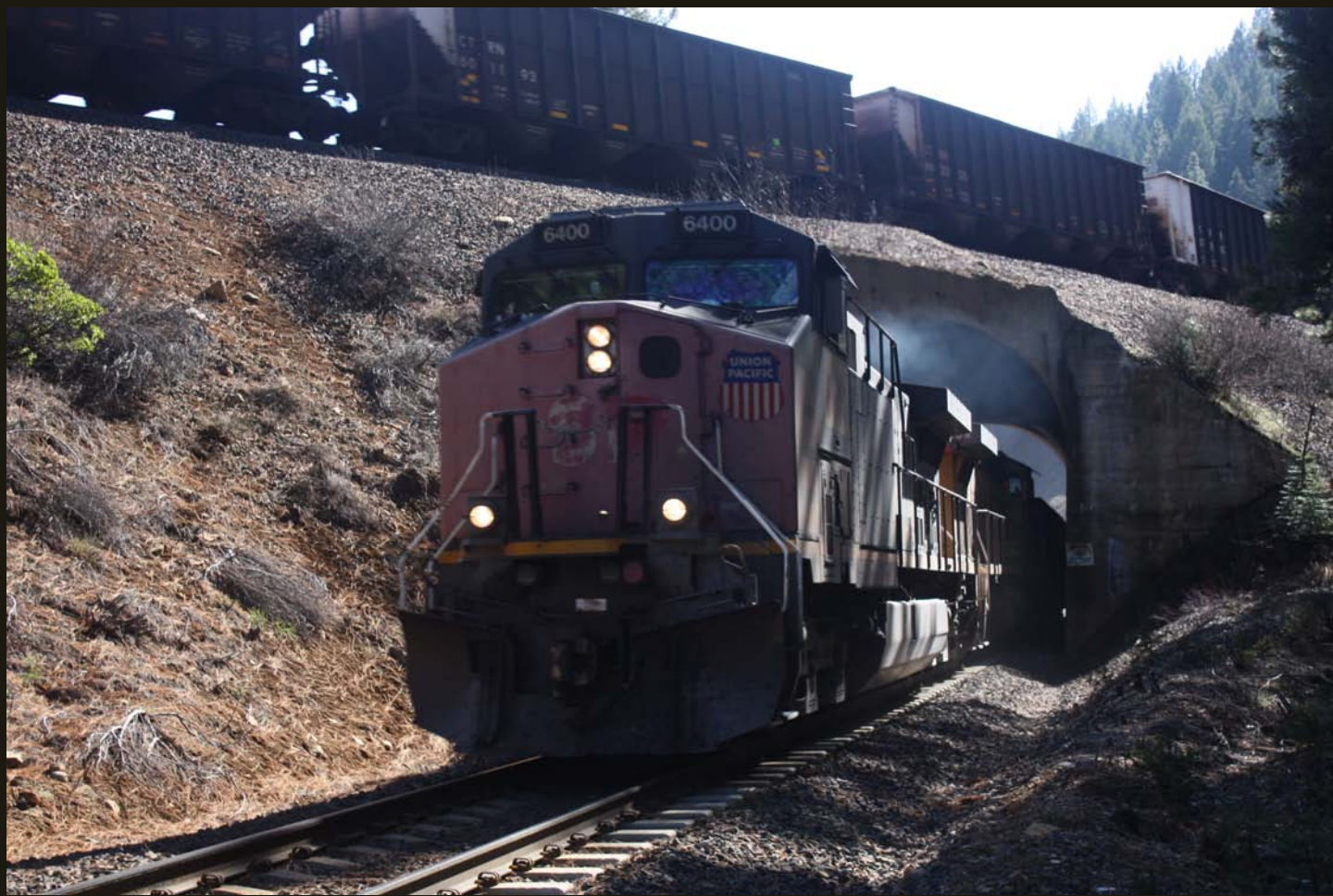
The container train passes under its own tail on the Williams Loop. The loop exists to create the elevation change in the photo.
