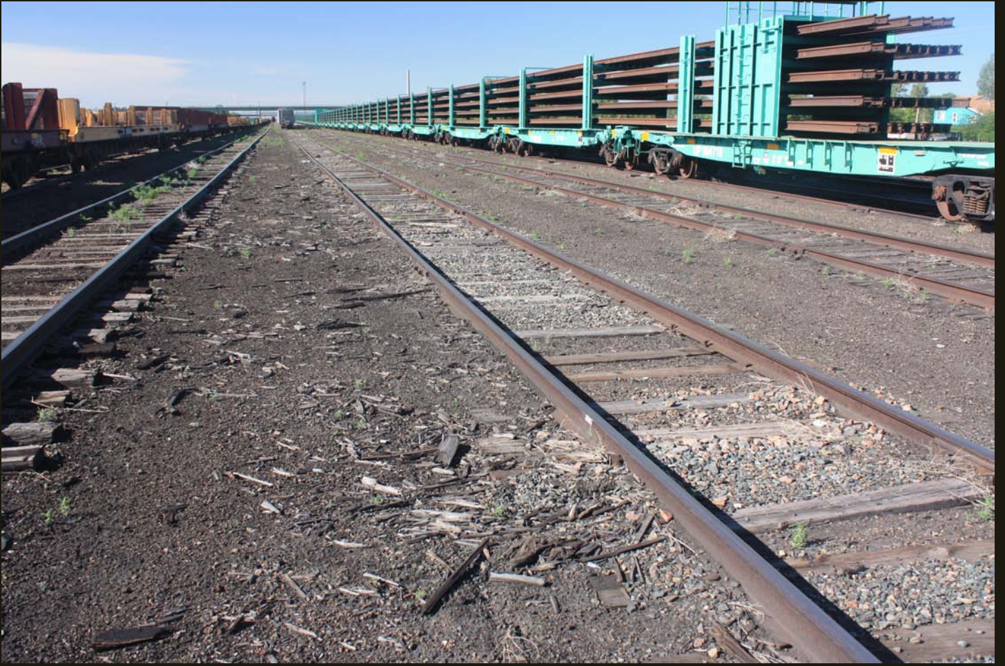
In UP's Laramie yard, a train of quarter-mile-long welded tracks awaits duty.
