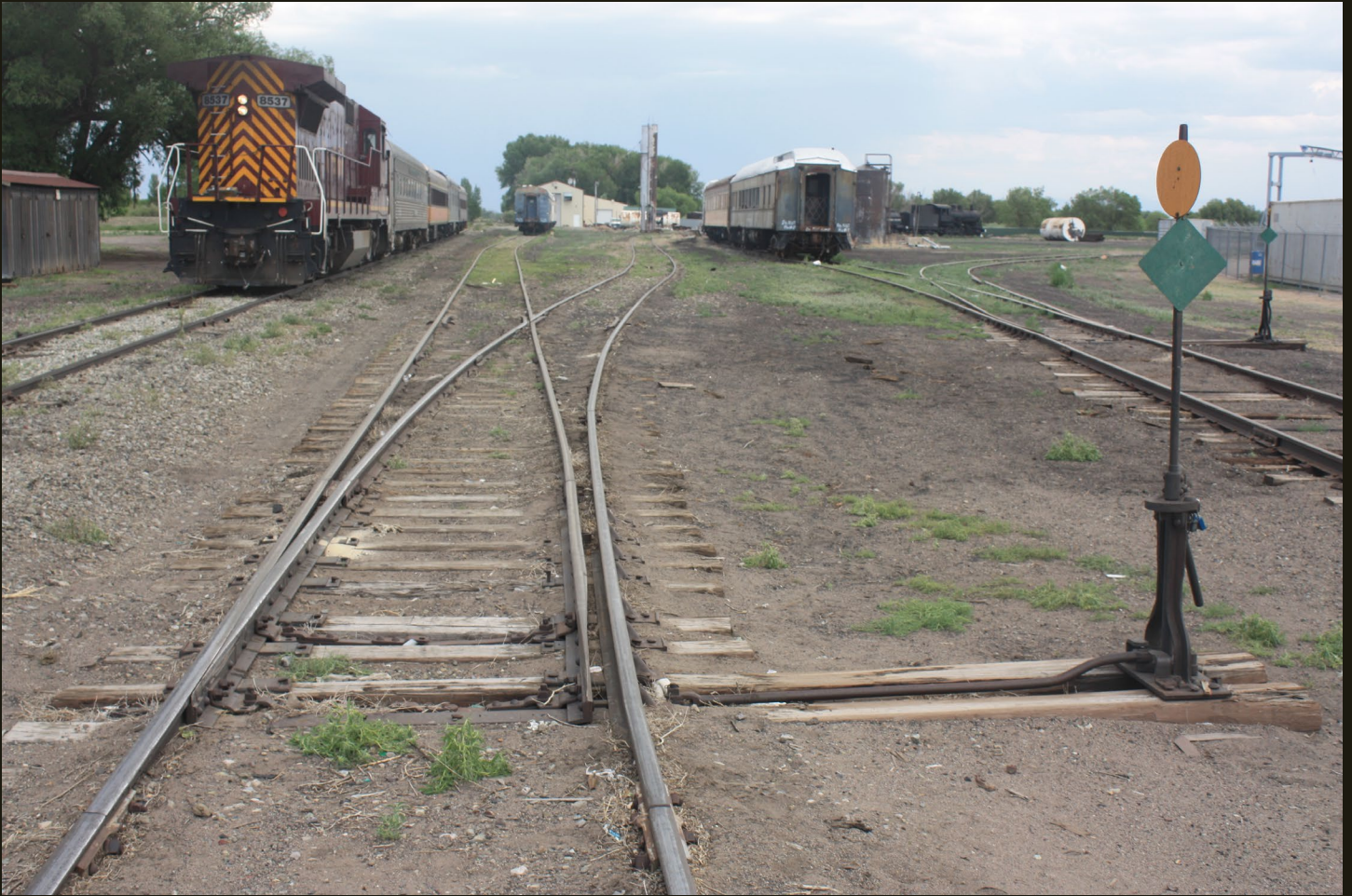
Another eastward view, a few steps north of the previous location; the passenger train on the left is the same as in the previous photo. There are three sidings to the right (south) of the mainline (with a passenger train). The rightmost siding has a switch with a curved track to the right, which is the west branch of a turning wye, now used for rolling stock storage. A steam engine is visible on the east branch of the turning wye.
