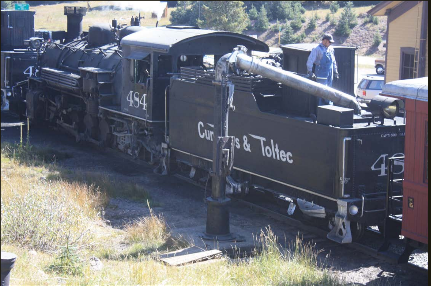
The second locomotive, the #484, gets watered first, with the lead engine still connected.
