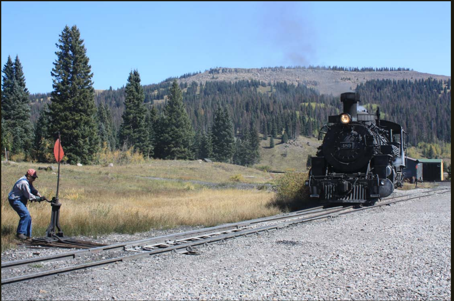
The lead engine has now turned at the wye and the switch is thrown to allow #489 onto the mainline, now heading west for the lonely trip back to Chama.
