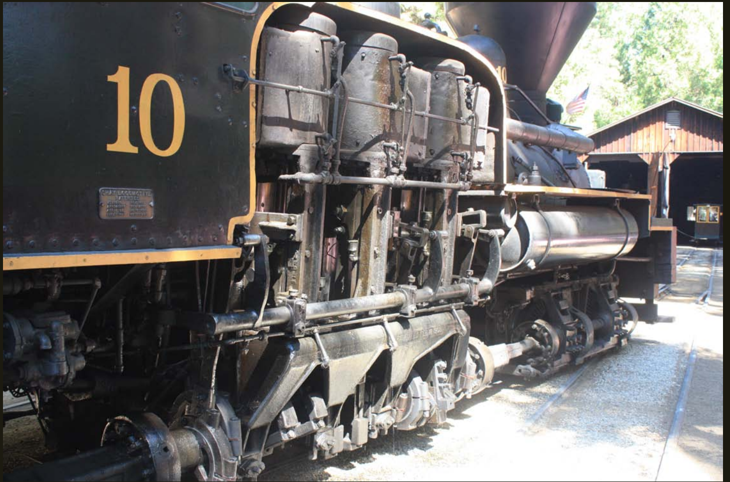
More detail of cylinders, pistons, and the horizontal drive shaft.
