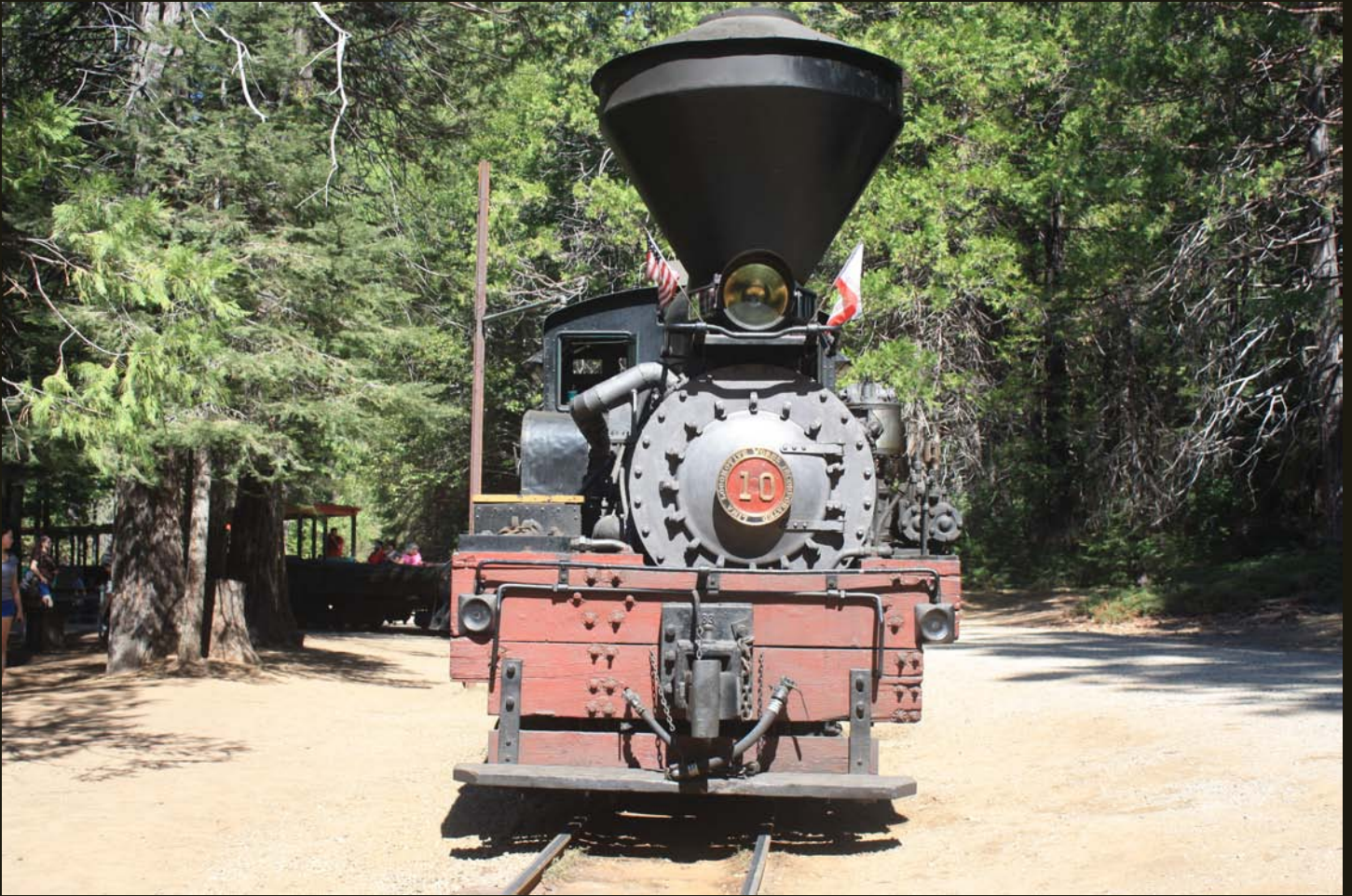
Shays ride asymmetrically on the track because of the side-mounted pistons.
