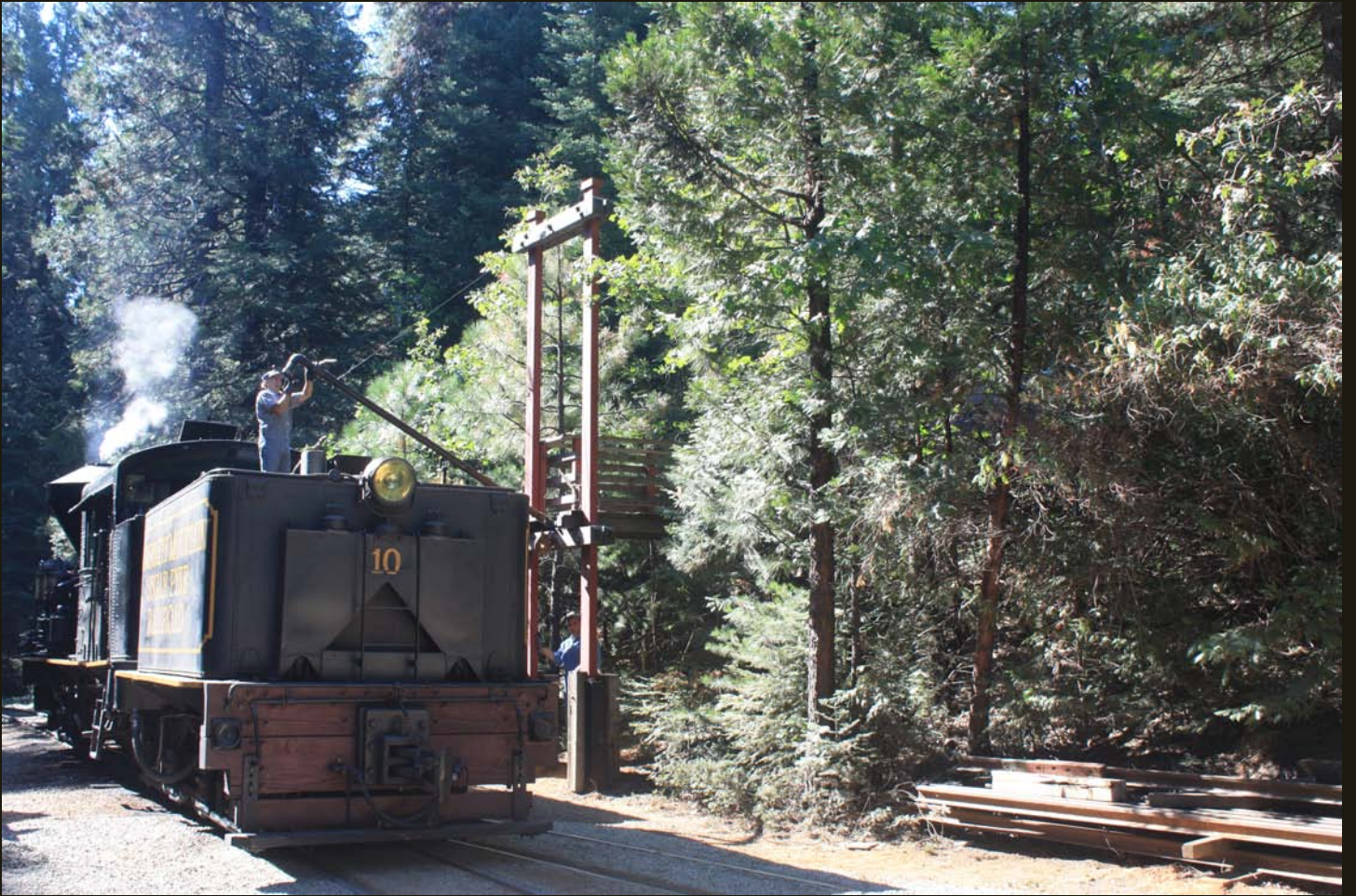
No. 10 burns oil, and its tender holds 1,200 gallons of oil and 3,420 gallons of water.
