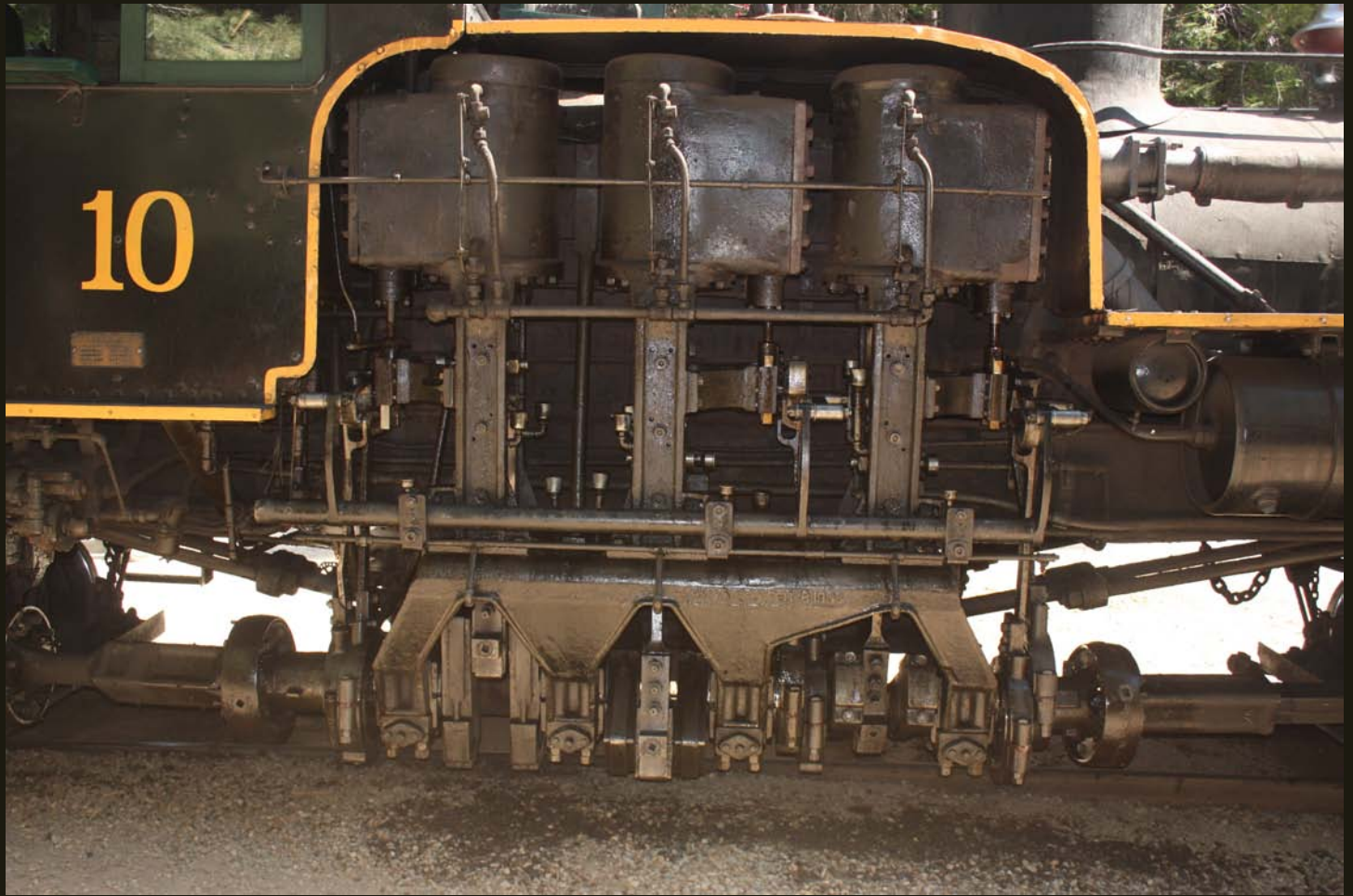
Detail of cylinders, pistons, and the horizontal drive shaft.
