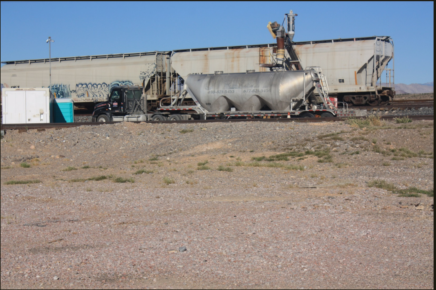
While I was there, a truck showed up to show us how the rail-to-track loading facilities work. I suspect they are loading silica sand. A topo map labels the sidings as “Moapa Siding.” The rail in front of the truck is the east branch of the wye for the SPLA&SL St. Thomas Branch (1912).
