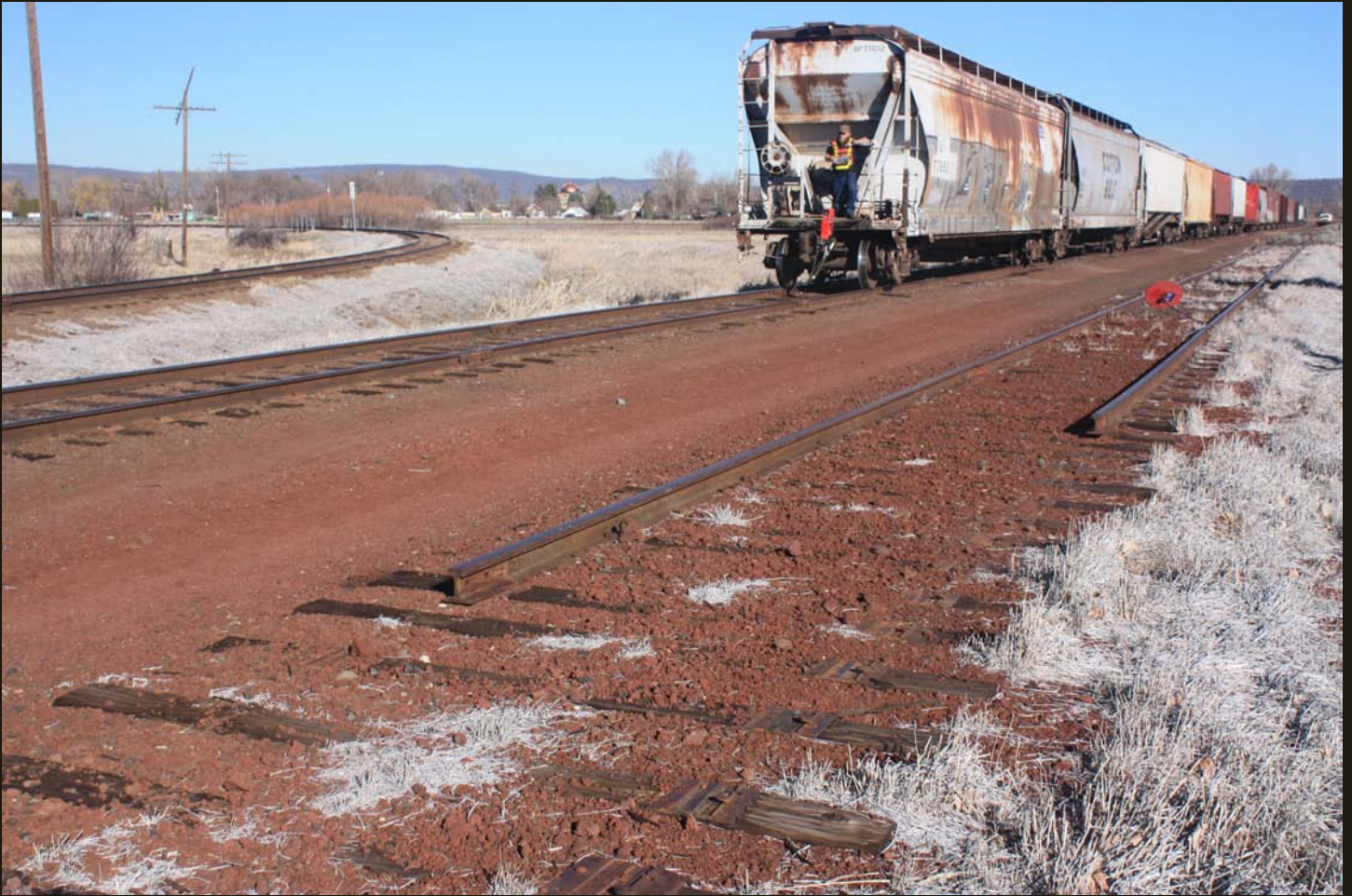
The LC train is now on the N-C-O grade and backing up to leave a few cars on the storage tracks south of the wye. The engineer is operating the train via remote control as he stands on the back of the train. Note the partially abandoned siding in the foreground.
