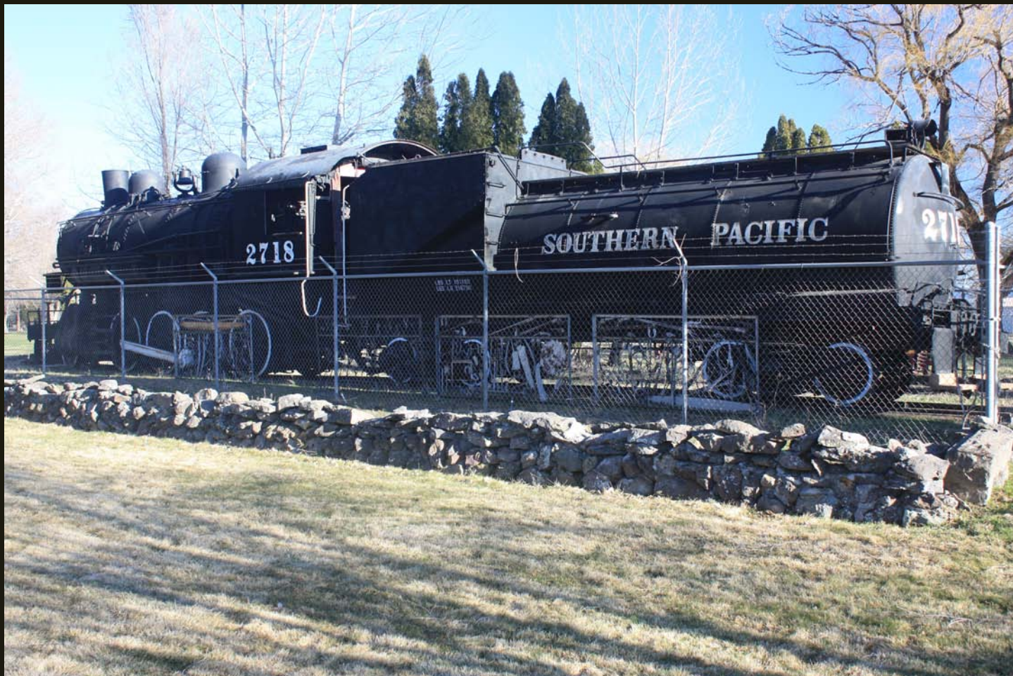
The Southern Pacific Railroad Locomotive #2718 is on display in Alturas. It was built by Baldwin in 1904 and donated to Modoc County in 1956. This locomotive was utilized on the Alturas to Reno route after standard gauging in the 1920's. Note the oil (not coal) tender, typical of the SP steam fleet, which had plenty of access to coastal California oil but virtually no access to coal.
