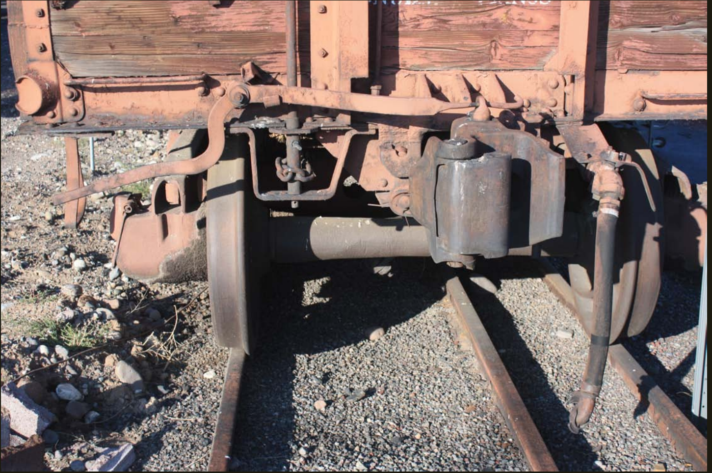
Dual gauge reached Antonito in 1901 and is preserved in the C&T (former D&RG/D&RGW) yard. I was thrilled to find dual-gauge rail still in place, with a parked standard gauge hopper.
