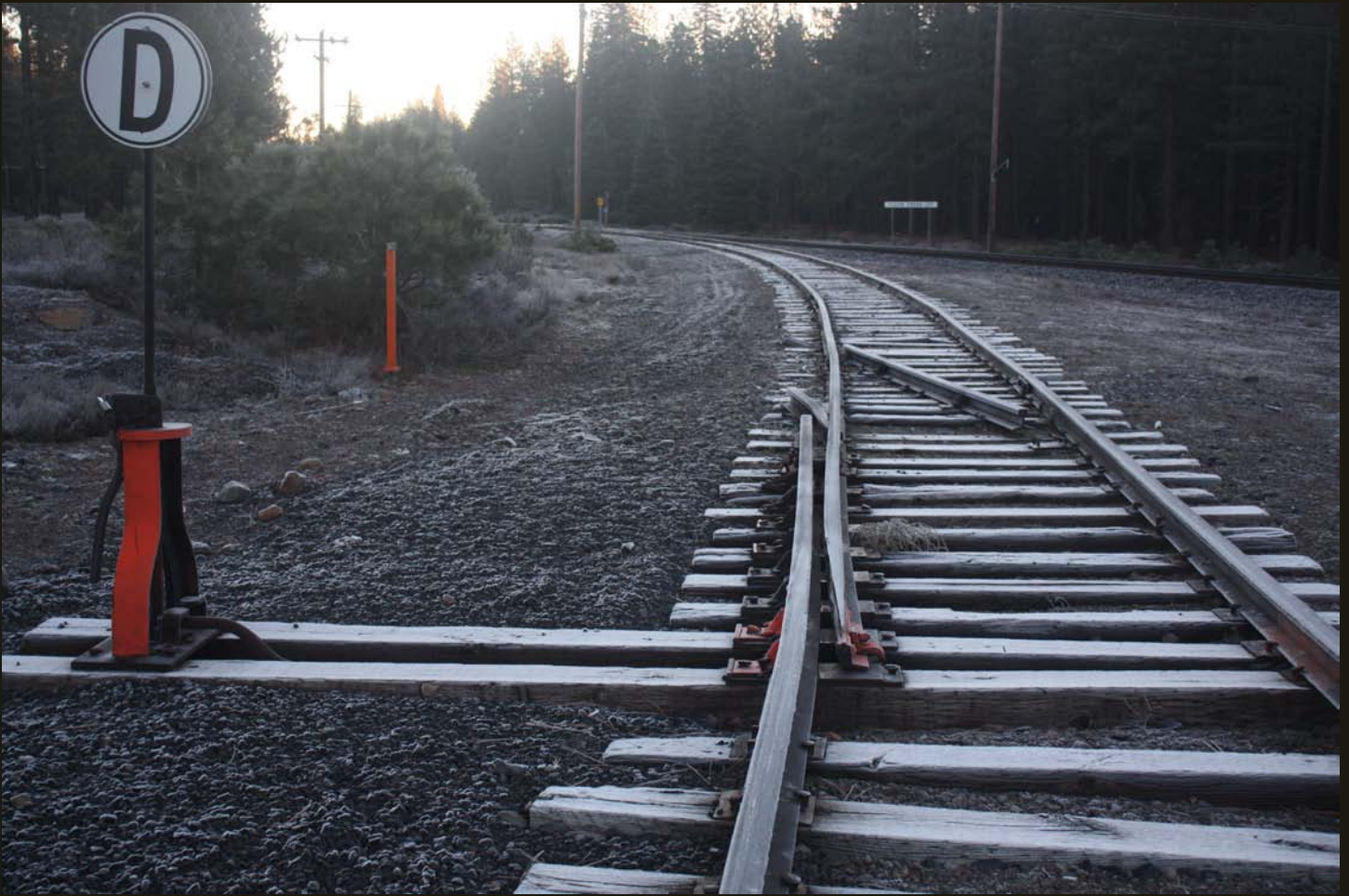
A quarter mile of rails on the Almanor Railroad remains for car storage, but no cars will go on or off with this switch setting. The rails west of the quarter mile car storage spur have been removed and no longer serve Chester.
