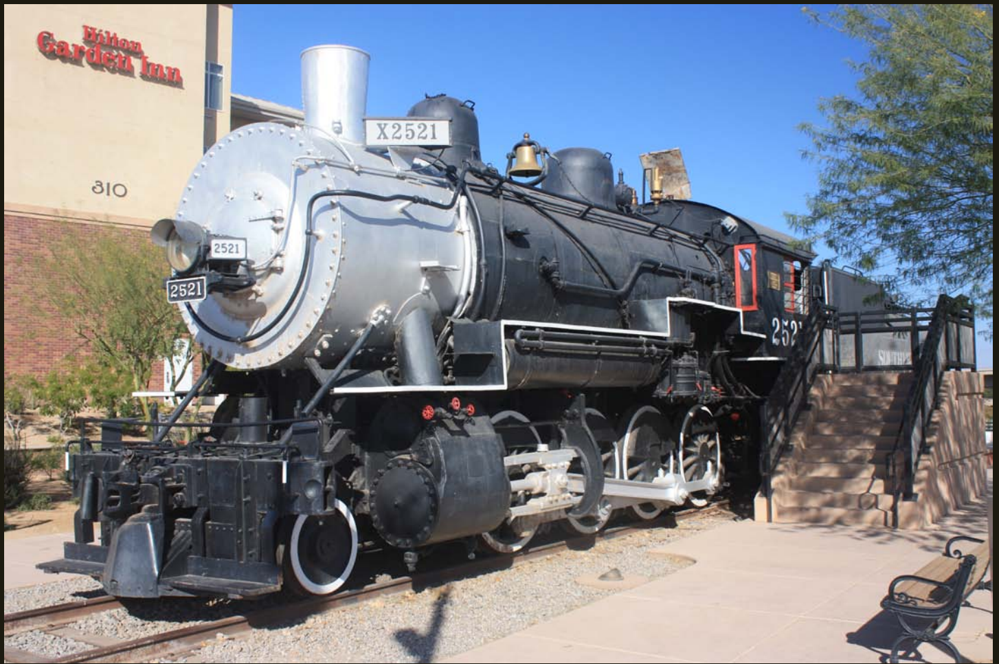
Southern Pacific Locomotive #2521 is on static display near the SP-YV wye. The 2-8-0 Consolidation-type engine was built by Baldwin Locomotive Works in 1907, placed in service by SP in 1908, and has since pulled passenger and freight trains an estimated 2.5 million miles around the Southwest.
