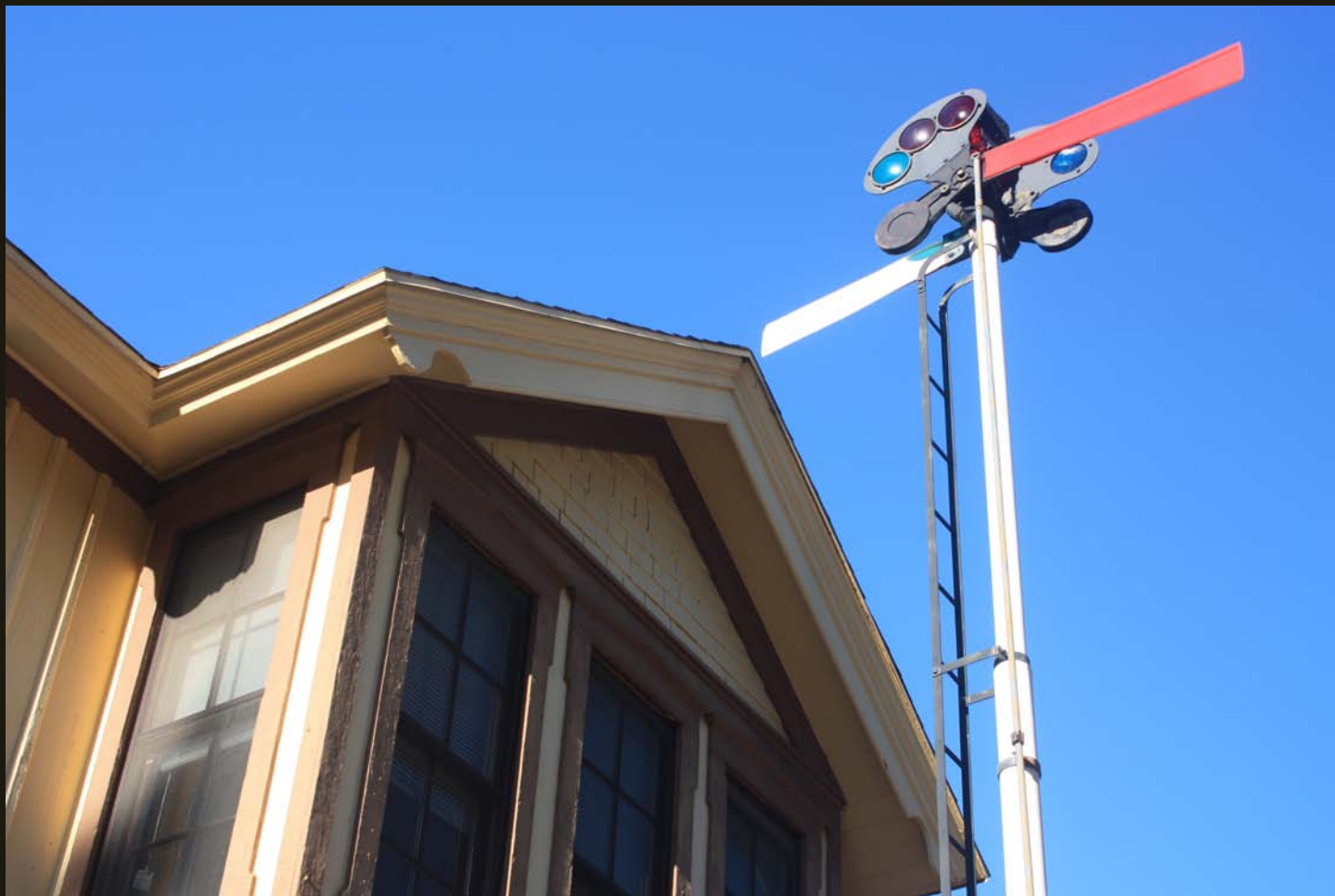
Train order semaphore on display at the Patagonia station.
