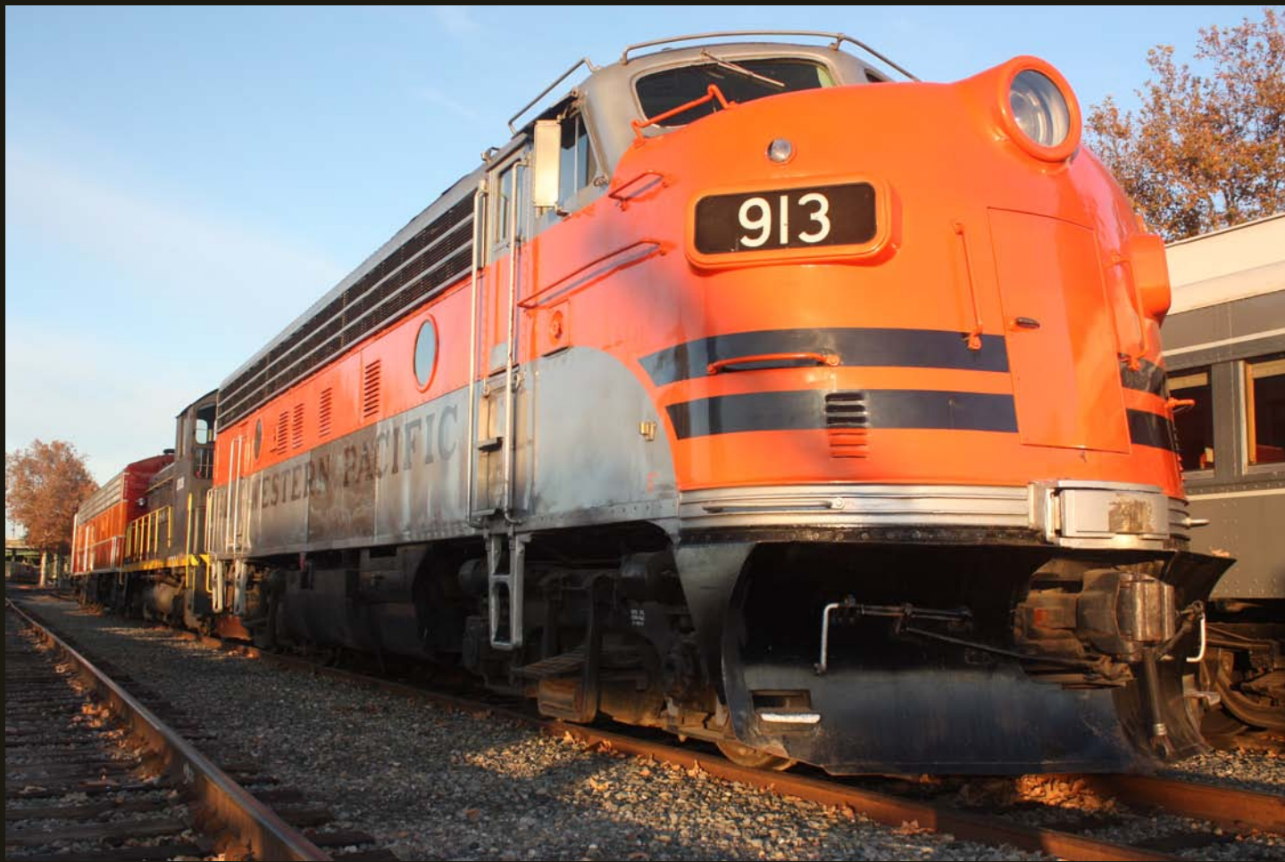
Northwestward view of the CP on the west side of the depot, where sidings display some of the California State Railroad Museum's rolling stock such as this Western Pacific EMD F7 diesel locomotive. (Note that this "Western Pacific" refers to the second Western Pacific Railroad, which was built in 1909.)
