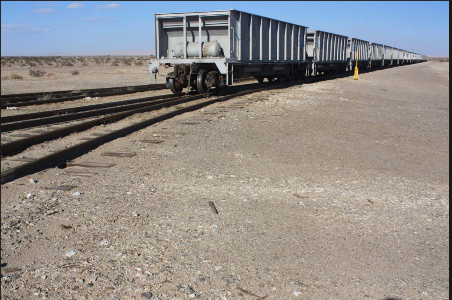
Another view of hoppers, showing a narrow gauge switch on an industrial railroad, a sight that can be seen nowhere else in the United States.
