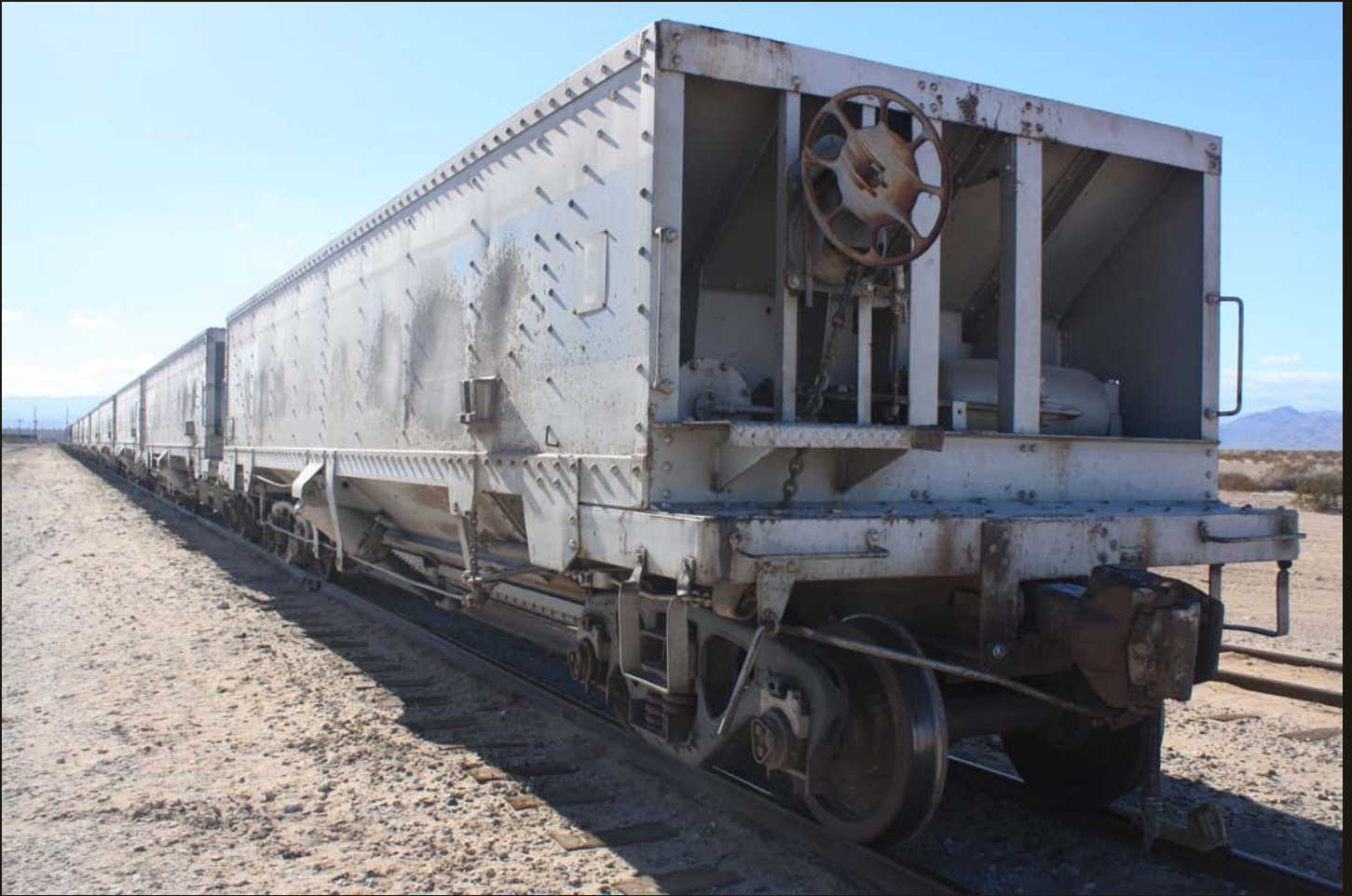
The narrow gauge of the tracks is obvious in comparison to the wheels, which appear close together (compared to standard gauge wheels).
