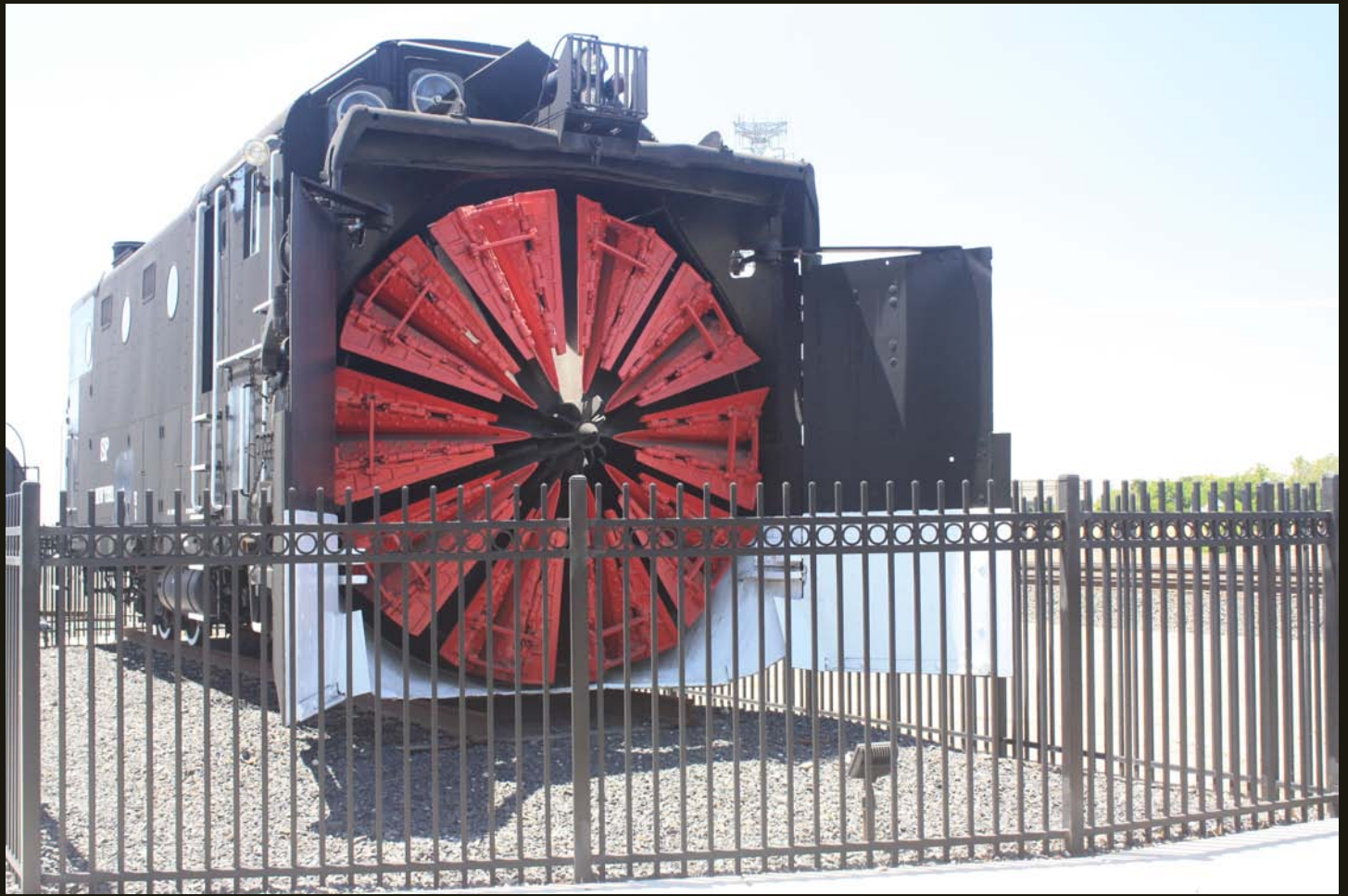
A SP rotary snow plow on display at the Roseville yard. Built in 1917, this unit cleared the line over Donner Summit until its retirement in the 1980's.
