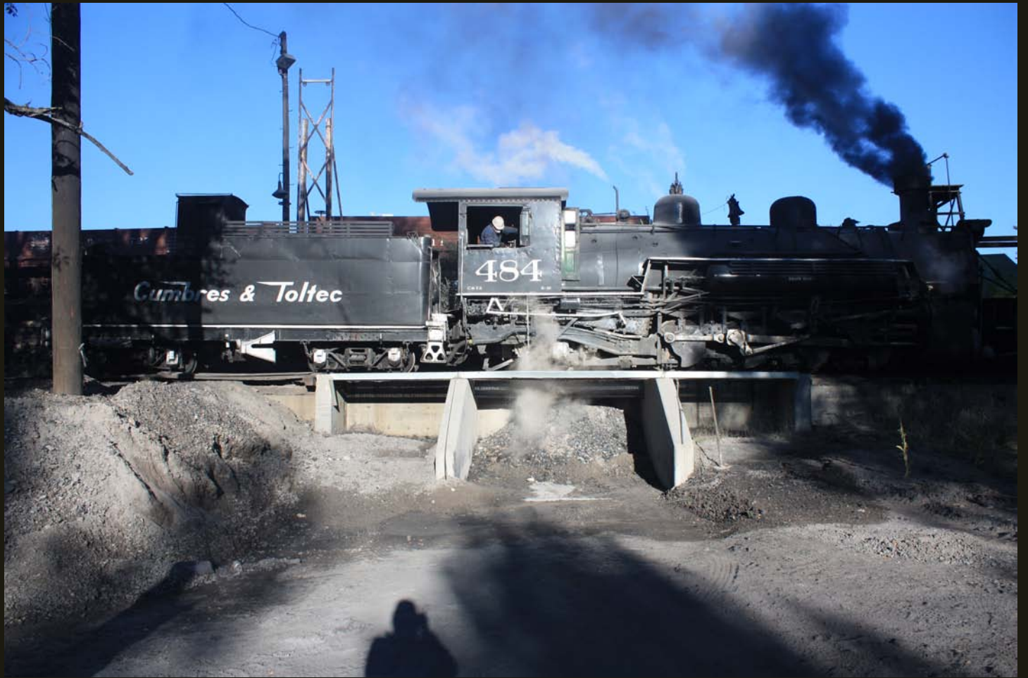
Dumping yesterday's coal ash, which cooled overnight.
