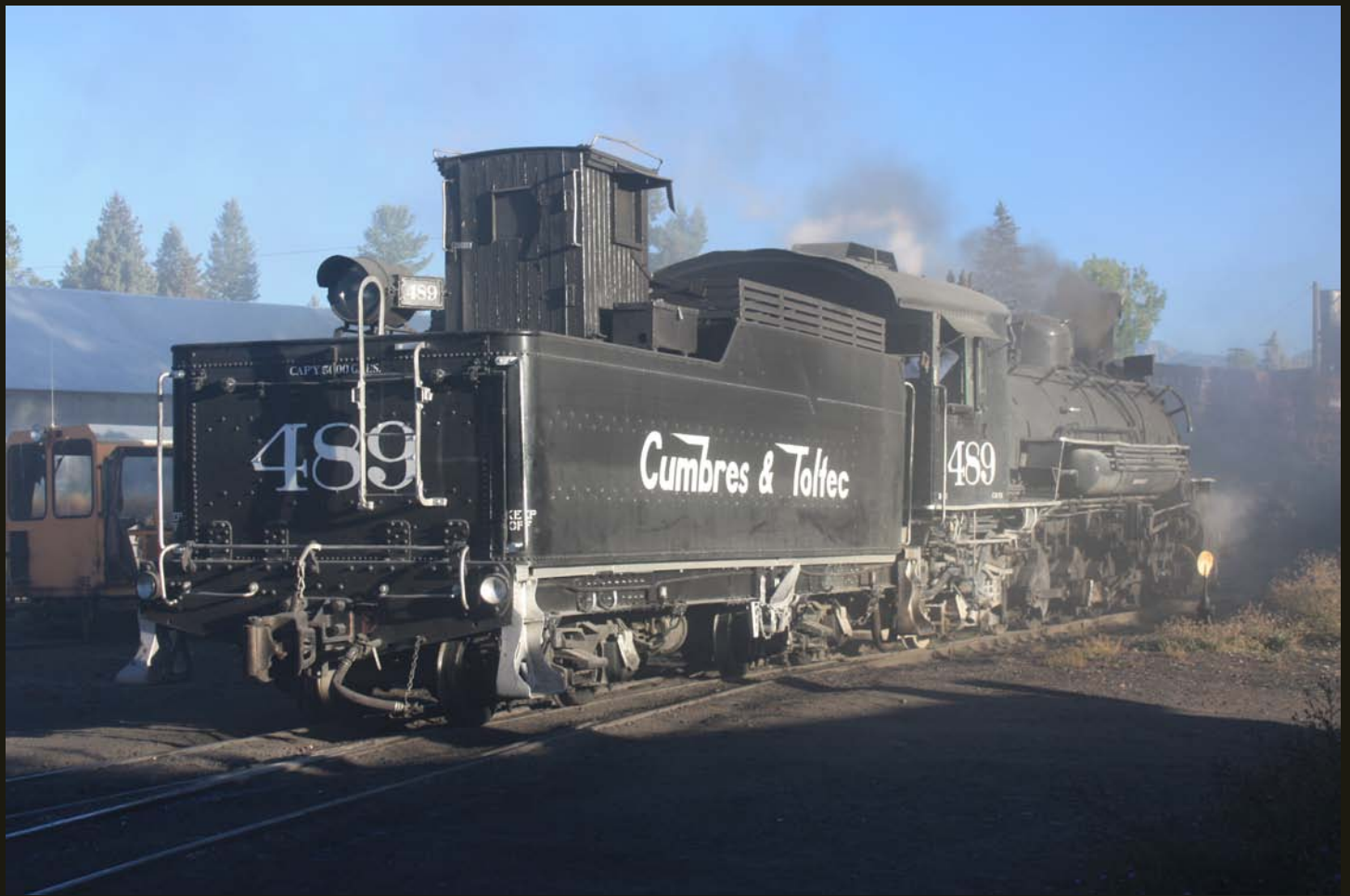
The tender will be filled with coal and water for the day's climb up to Cumbres Pass.
