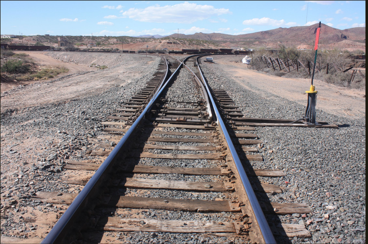
Northwest view of the Rincon wye; the RGM&P (1881) line to El Paso is in the foreground. The curve to the right heads north to Santa Fe and the curve to the left heads to Deming and the connection with the SP Sunset Route (1881).
